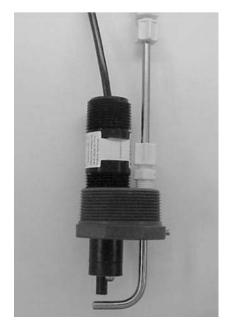
The Jet Spray Cleaner eliminates routine manual sensor maintenance by cleaning Model 399VP with water or compressed air. Flow through the cleaner can be controlled by a solenoid valve. (Model 399 with integral cable shown)
